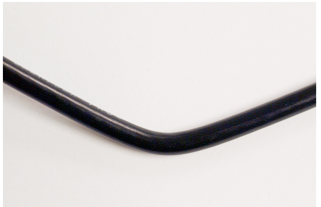
A BREAK ON THE CABLE
