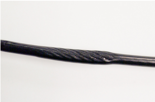
"NECKING", STRECHED CABLE COVERING
