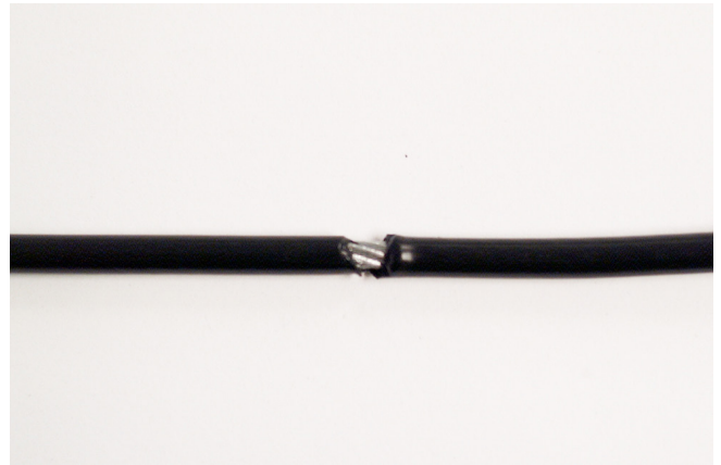
A CRACK IN THE CABLE COVER
